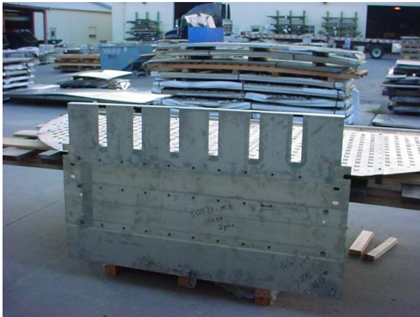
Figure 6 – Example of a proper opening spread for a highly blocked weir
