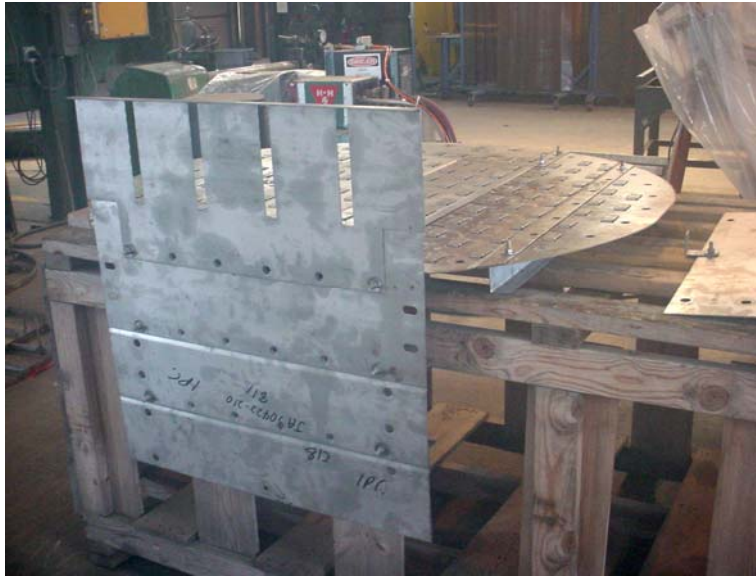
Figure 5 – Example of a proper opening spread for a highly blocked weir
